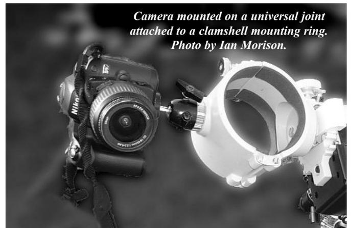
*Camera mounted on a universal joint attached to a clamshell mounting ring. Photo by Ian Morison.*
