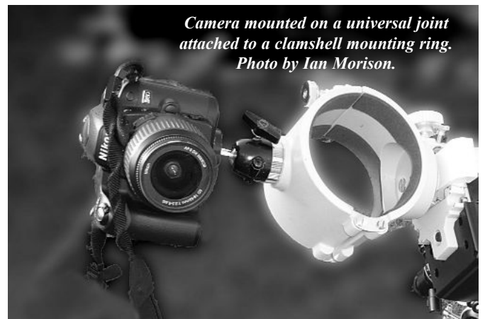
Camera mounted on a universal joint attached to an equatorially mounted driven telescope, allowing any part of the sky to be tracked. Photo by Ian Morison.
